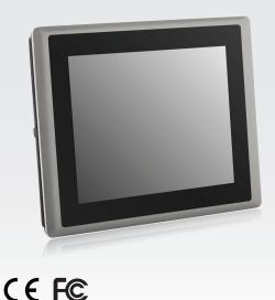
12.1" TFT XGA 4:3 Display Module with Resistive 5-wire / Projected Capacitive Touch
