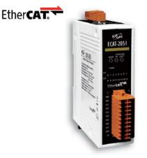
Features On the fly processing: EtherCAT Powerful MCU handles efficient network traffic 2 x RJ-45 bus interface Distance between stations up to 100 m (100 BASE-TX) Support daisy chain connection EtherCAT conformance test tool verified Removable terminal block connector LED indicators for the input status Built-In isolated 16 digital inputs RoHS compliant ESD Protection 4 KV Contact for each channel CE FC X RoHS
