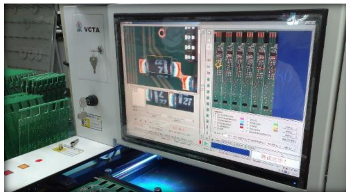
Soldering Inspection System – Image Processing
