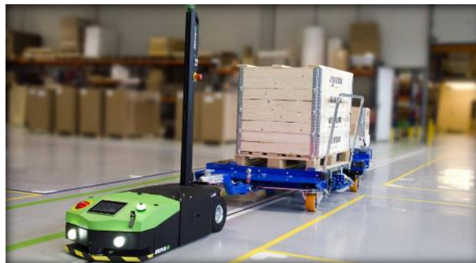
Automated Guided Vehicle – Power Supplied by Battery
