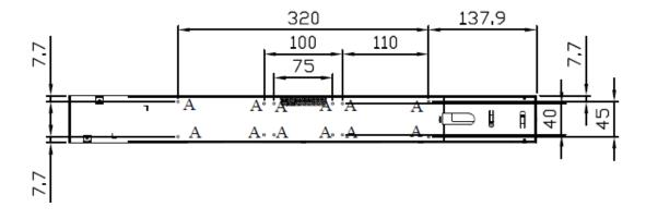
Note : O.D : Outline Dimension B.O : Bezel Opening A.A : LCD Active Area A:12-M3\_USER HOLE\_MAX DEPTH=3mm
